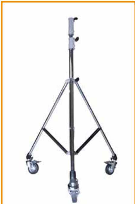
Stand 2 sec. alu silver 114-200cm Ø35mm with wheels, suitable for Maxi Boom.
